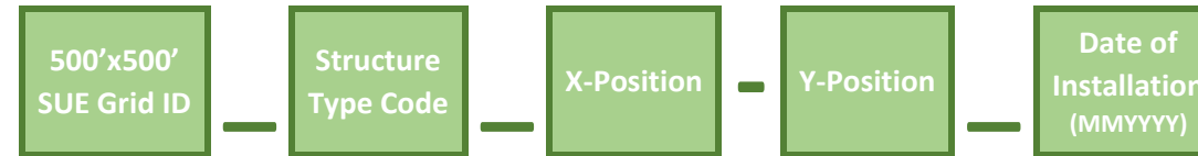
Figure 1D.3.3.3, Structure ID Format
