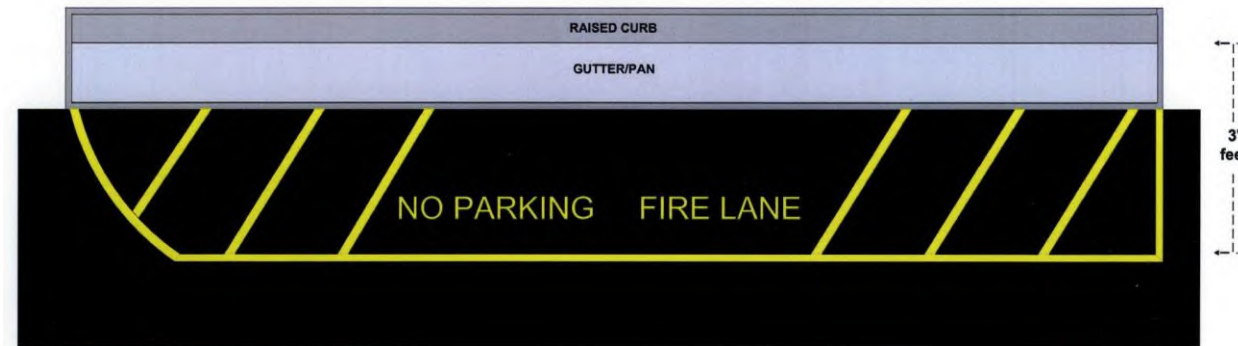
Figure 3.1.16.3-1 – Fire Lane Curb Marking
