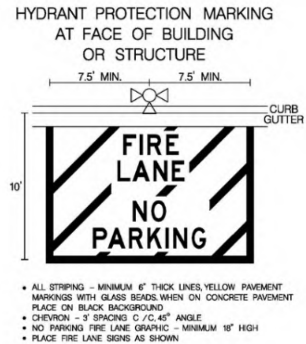
Figure 3.1.16.4-1 – Fire Lane Markings at Hydrants
