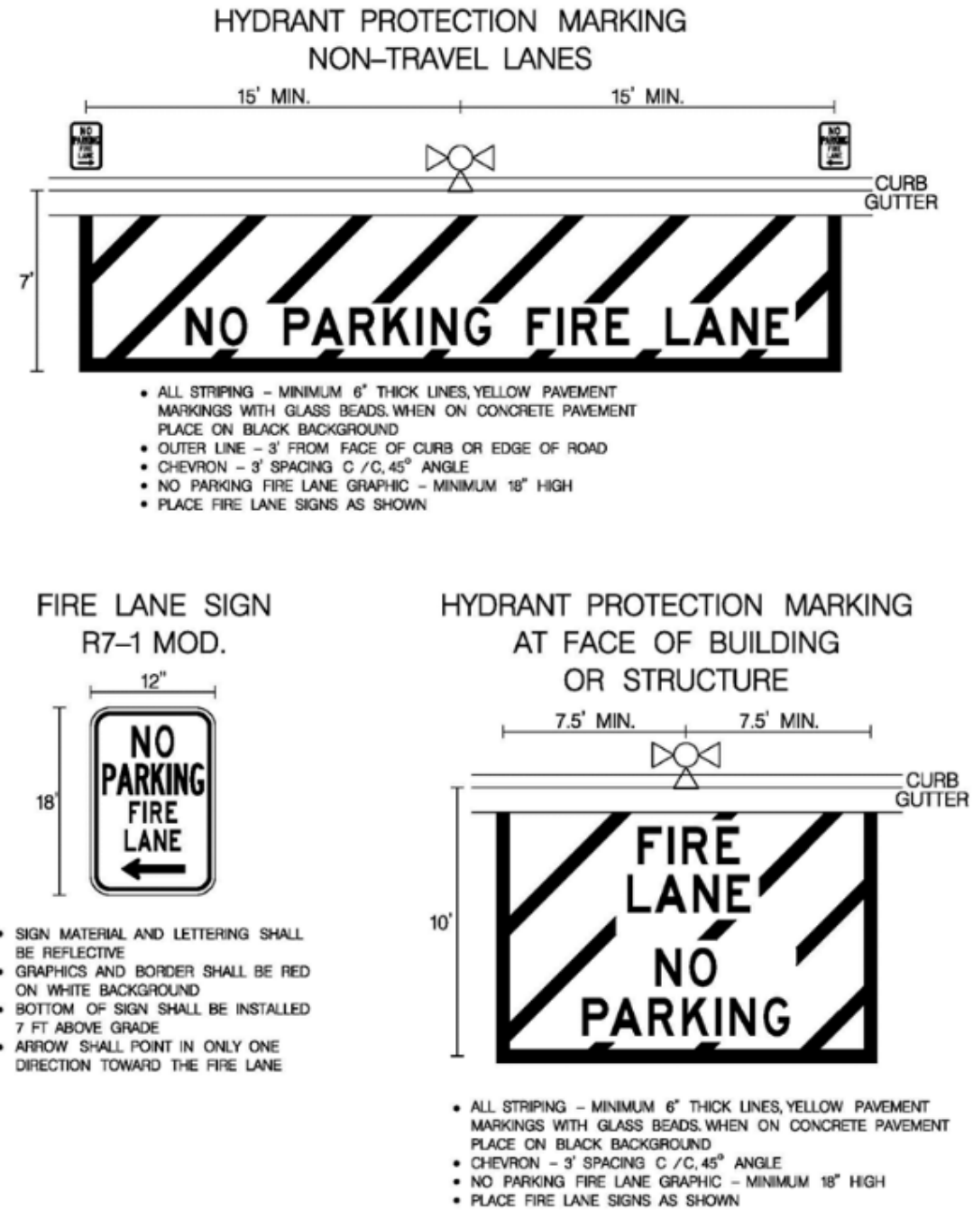
Figure 3.1.16.4-1 – Fire Lane Markings at Hydrants
